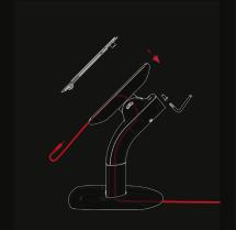
Unscrew top bracket that holds the adhesive and remove. Feed cable through the stand.
