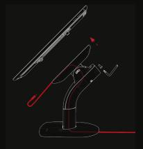
4. Re-attach top bracket and secure with the lock screw.
