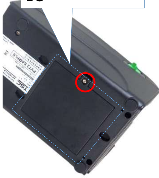
RTC connector (dotted line: Wireless connector position)
