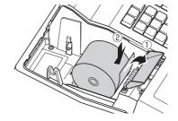
3. Insert the paper straight into the paper inlet, and press 1. The paper then feeds through and appears in the print area.
