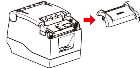
C. Turn the white gear on the cutter, and take jammed paper out.
