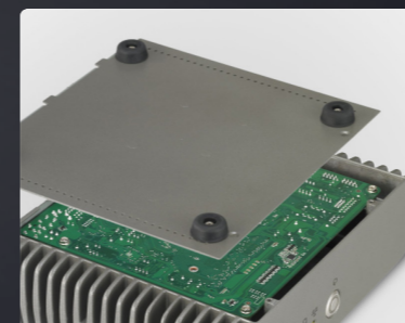
The motherboard is easily accessible for efficient upgrades.
