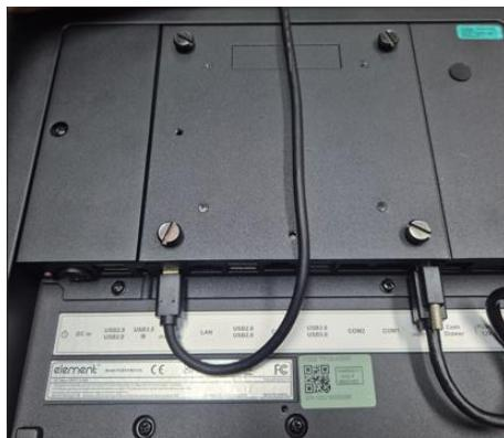
Align the FEDP cable with the notch on the back of the stand then reattach the stand
