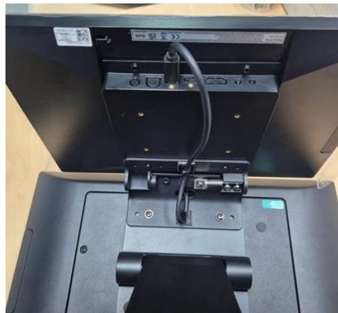
Feed the cable in to the correct length and position then attach to the plastic clips
