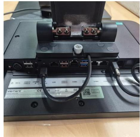
Feed the cable through the hole in the top of the CDU bracket then attach the connector plug to the port on the CDU
