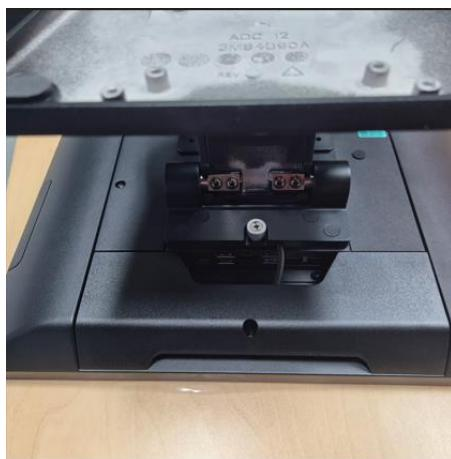
Connect the FEDP cable to the terminal and lay it across the back of the screen
