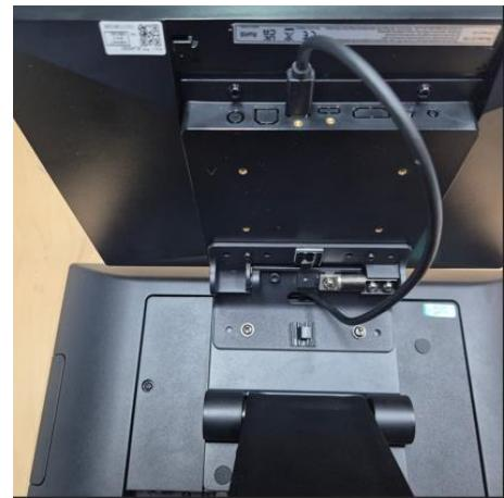
Remove the rubber covers from the screw holes in the back of the stand then attach the CDU with the 2 supplied screws.
