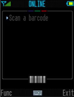
To press “**Func**” (L key), you are able to view the scan logs and configure the display option.
