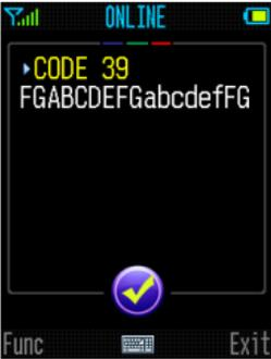
For more Reliable Data Transfer, the useful Host Acknowledgement function provides a helpful handshaking protocol to ensure the scanned data is successfully received by host application. Once this function was enabled, the scanner will wait for an **ACK** or a **NAK** message issued by the host application after each scan. And the scanner can not scan any barcode before it completes the handshaking process.
