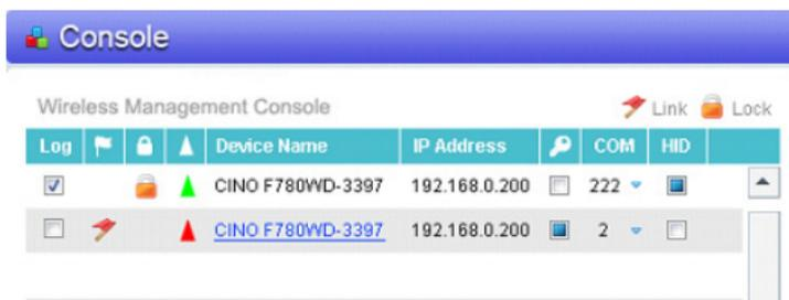
By default, each connected Wi-Fi scanner work as a local serial device of your remote host. You are able to design your application without involving complicated TCP/IP (socket) programming. This is helpful for your application to work with multiple scanners.
