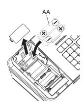
**4** Replace the battery compartment cover. Please make sure that the battery compartment cover is fastened securely with a click sound.
