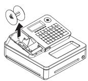
**3** Remove the battery compartment cover and install two new "AA" type manganese batteries in the battery compartment over battery extraction ribbon.
