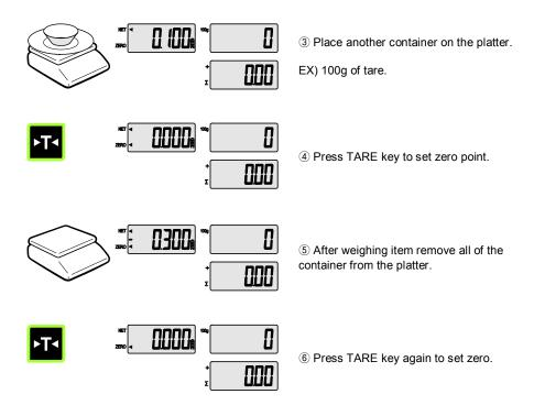
• NOTICE: To remove TARE funtion press "TARE" Key again after removing the container from the paltter. Automatic tare clearing function may not be applied to all of PR series.
