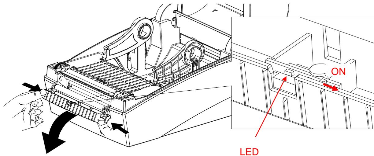
3) Remove one sheet of the label paper, and insert the paper as shown in the image below.
