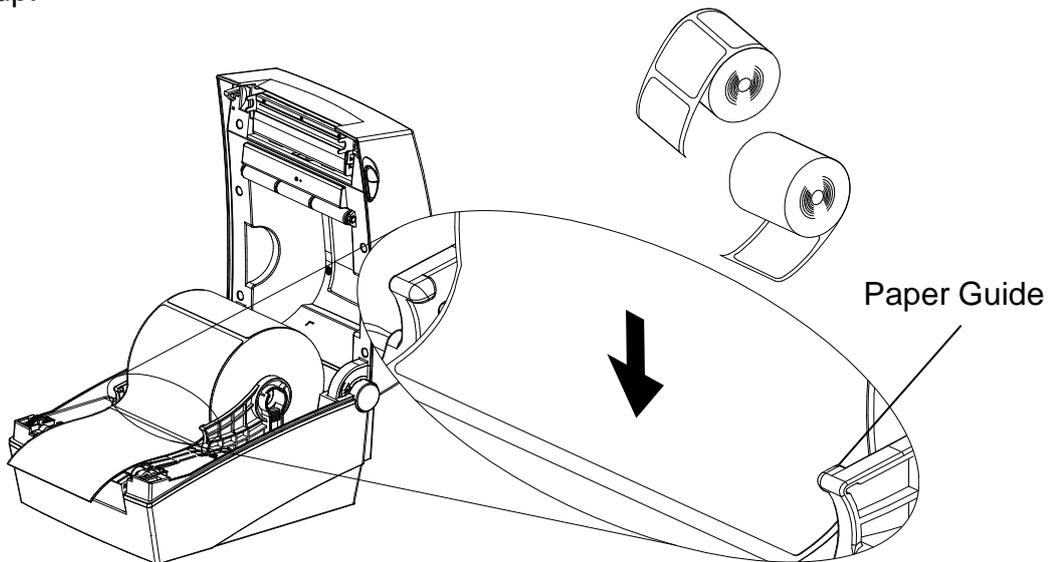
4) If you use Black-Mark or Notch paper roll, please lift up the paper and match the sensor position adjust the black mark or notch hole.
