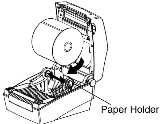
3) Pull the paper so that it extends out of the front of the printer. Push the paper under both of the Paper Guide.
