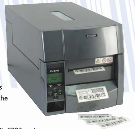
For specialist applications, the CL-S703 and CL-S703R models print at 300 dpi making them ideal for small labels with 2D matrix barcodes such as Datamatrix, Codabar, QR-Code and PDF417. The higher resolution 300 dpi is also ideal for serial number rating plates featuring company logos and idents like CE or WEEE logos or where intricately designed fonts are required.
