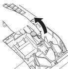
3 Note the (+) and (-) markings in the battery compartment. Load a set of two new "AA" type manganese batteries so that their plus (+) and minus (-) ends are facing as indicated by the markings.
